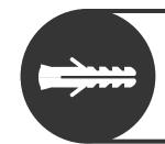
When there is no stud or support for the screw, use the provided drywall anchors
